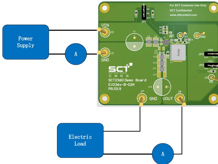
**Figure 1. SCT2360EVM Power Supply, Load and Measurement Equipment Setup**
