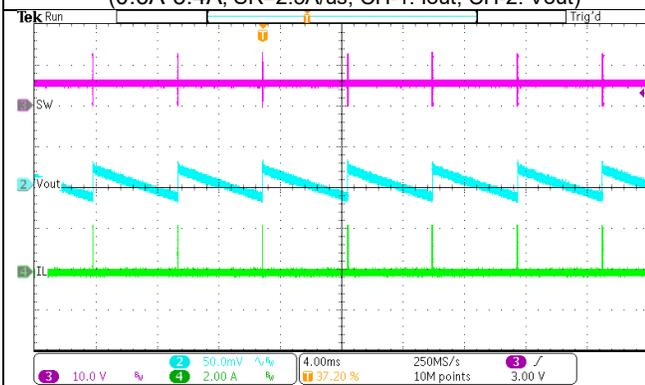
Figure 14. Switching Waveforms and Output Ripple in PSM
