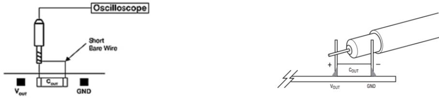
Figure 2. Measuring Voltage Ripple Across Terminals or Directly Across Ceramic Capacitor
