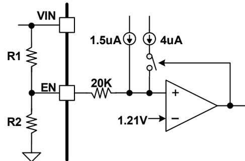
Figure 16. VIN UVLO Programmable by EN Divider
