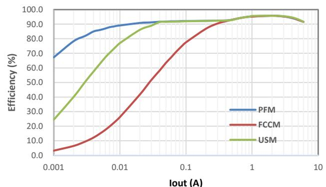
SCT236X Buck Efficiency, V<sub>IN</sub>=12V, V=5V, 400kHz
