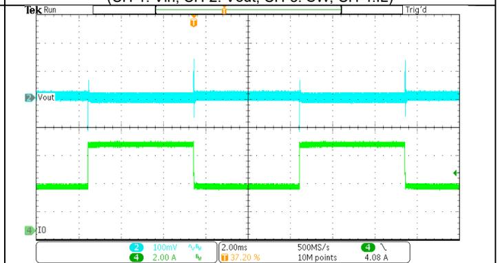
Figure 13. Load Transient
