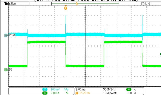
Figure 12. Load Transient
