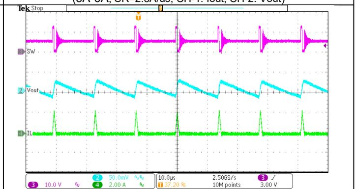
Figure 15. Switching Waveforms and Output Ripple in USM
